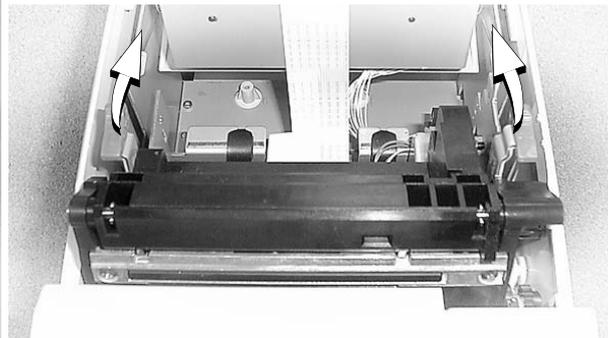
3. Insert the ribbon cartridge into the printer. You can see a properly installed ribbon in the illustration below with the arrow pointing to the knob.
