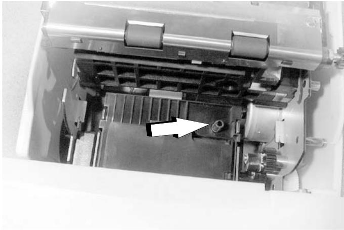
4. Turn the knob two or three times to make sure that the ribbon is seated correctly.
