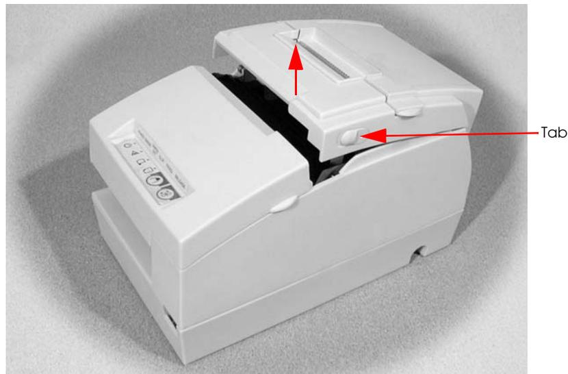
Push the levers backward to open the unit as shown below, and then remove the jammed paper.
