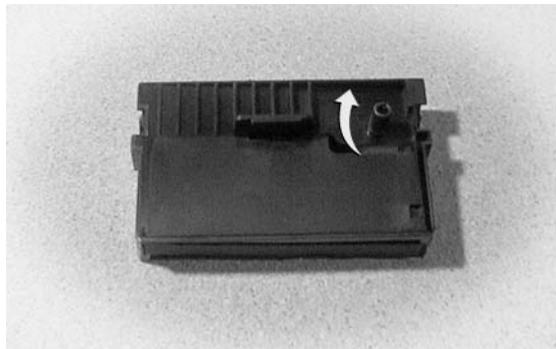
2. Open the unit cover, as shown below. Inside the printer, push the levers backward to open the unit.
