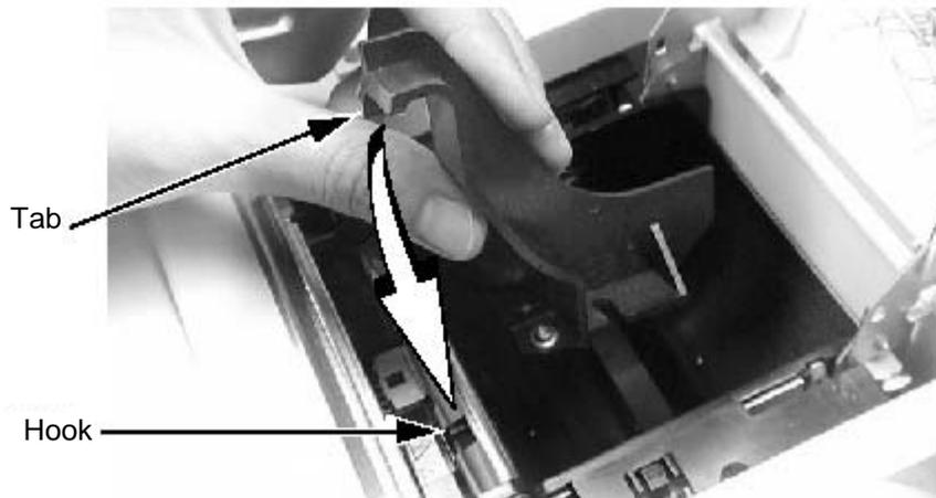
When using 58mm paper, slide the entire paper guide to the left; when using 60mm paper, slide the entire paper guide to the right. Make sure that the paper guide is set securely in place.
