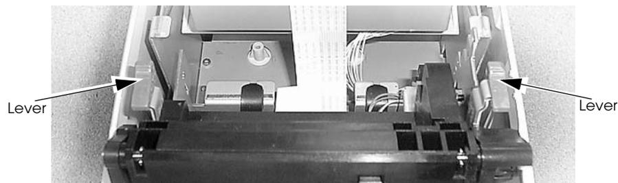
If the paper roll cover cannot be opened because paper is caught in the autocutter in the receipt section, follow the instructions in the autocutter section below.
