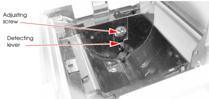
3. Tighten the adjusting screw, and check to be sure that the detecting lever moves freely.
