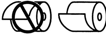
6. Pull out a small amount of paper, as shown. Then close the cover and tear off the extra paper by pulling it toward the front of the printer.
