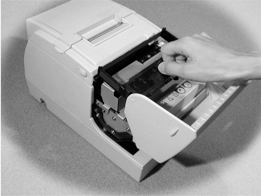
5. Turn the knob two or three times to make sure the ribbon is seated correctly. You can also look at the side of the slip unit to see if the ribbon is in the correct place. See below.
