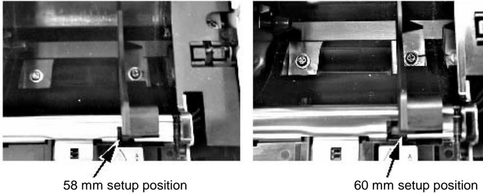
Secure the paper guide in place with the screw that was provided with the paper guide.
