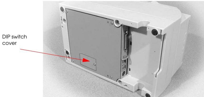
3. Set switches using a pointed tool, such as tweezers or a small screwdriver.
